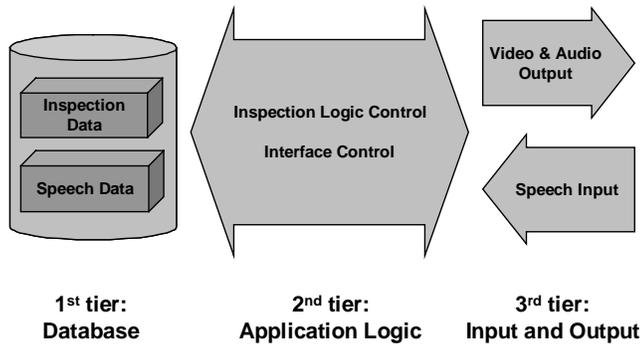
**Figure 4:** This figure shows the three tiers of the software architecture. The Control Tier sits between the input / output components and the data structure for the inspection data and the speech data.
