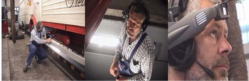
**Fig. 3.** Xybernaut<sup>®</sup> MA<sup>®</sup> IV used in a speech-controlled automotive inspection
