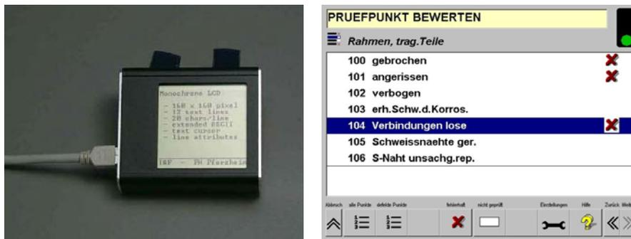
**Fig. 1.** Examples for small display (12 lines, 20 char.) and GUI design with traffic light symbol
