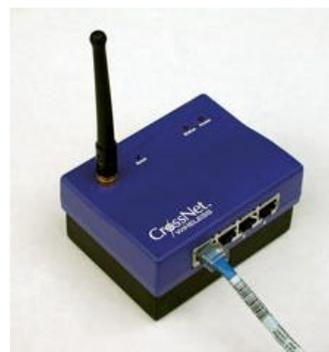
**Figure 4b:** Bluetooth-enabled sensor (Crossbow)
